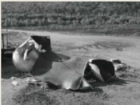
Vessel flattened on ground following BLEVE. iii
