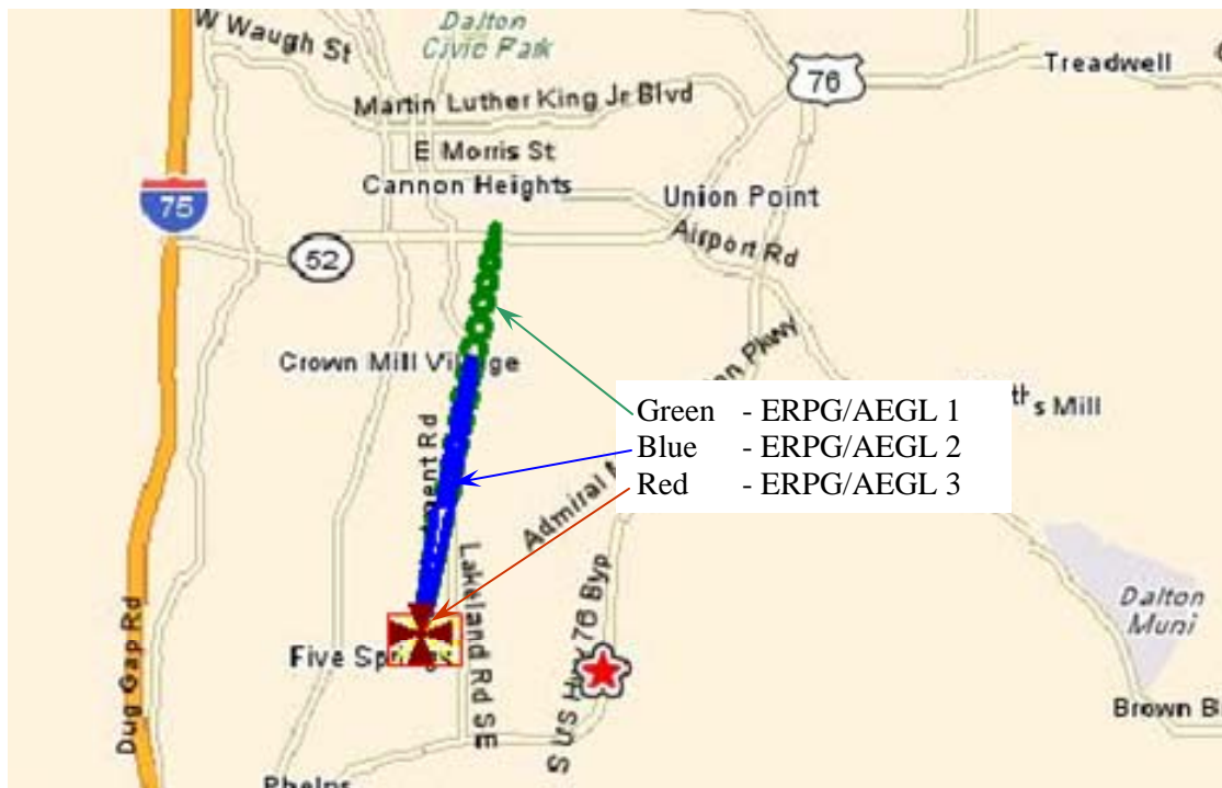
Figure 4. Predicted hazard zones for the manway gasket release.
