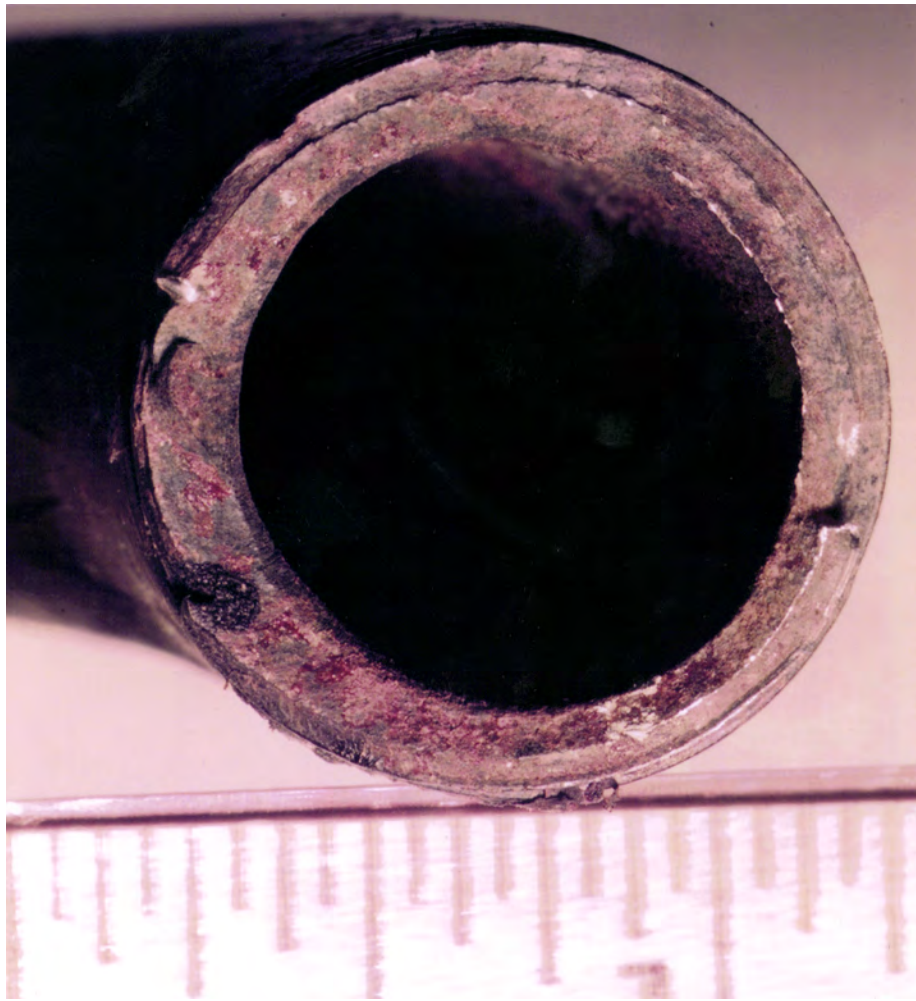
Figure 37 View of the fracture surface of the one inch pipe (A1) which carried liquid propane to the vaporizer unit
