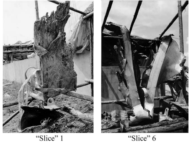
Fig. 6. Vaporiser remains, reassembly.
